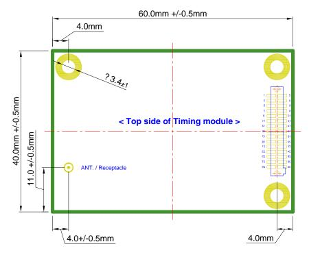
Board to Board connector: SFC-115-T2-F-D-A(2x5, 30 Pin)
