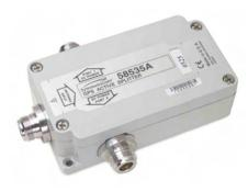
An antenna splitter may be used to drive multiple GPS receivers using a single antenna. With built-in amplification to overcome splitter losses, the Active Splitters may be conveniently cascaded without adding separate amplifiers and bias-tees between splitters. Power is conveniently obtained from the GPS receiver(s) connected to the amplifier, eliminating the need for a separate dc power supply and wiring.
